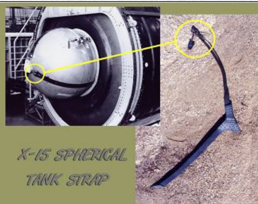
X-15 SPHERICAL TANK STRAP THIS TITANIUM STRAP WAS USED TO SECURE A SPHERICAL TANK OF HELIUM, WHICH WAS SIMILAR TO THE TURBOPUMP FUEL TANK PICTURED ABOVE. THE HELIUM WAS USED TO PURGE OTHER GASES FROM THE XLR-99 ROCKET ENGINE. CIRCLED IS ONE OF THE THREE ADJUSTABLE FASTENERS THAT JOINED THE STRAP TOGETHER
