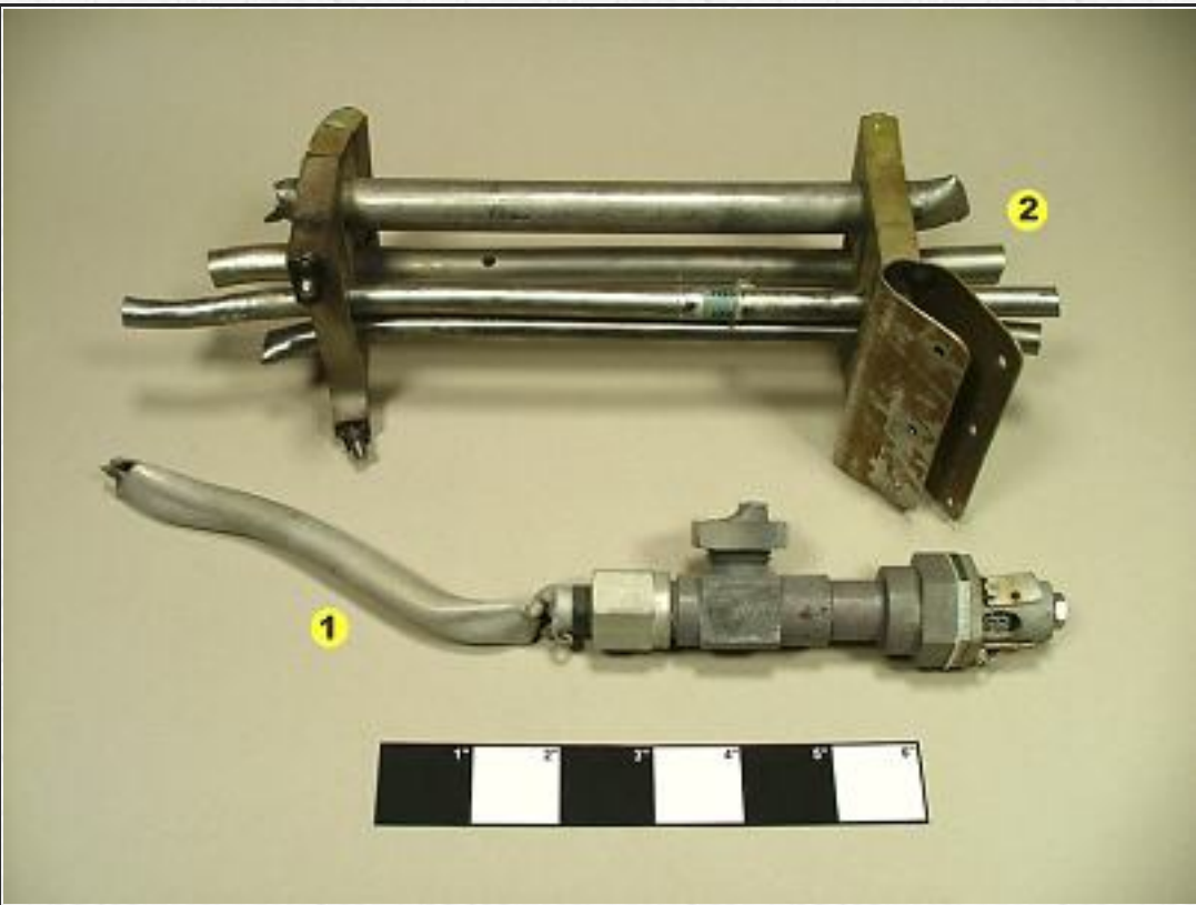
X-15 PIPE BUNDLE & VALVE 1. AIRCRAFT NITROGEN SYSTEM PRESSURE RELIEF VALVE 2. TUBING BUNDLE AND GUIDES. NOTE PARTIAL HYDROGEN PEROXIDE IDENTIFICATION LABEL ON FOREMOST TUBE.
