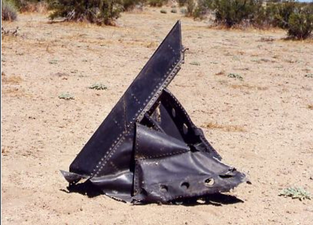
X-15 HORIZONTAL STABILIZER SECTION THIS IS THE FORWARD CENTER SECTION OF THE X-15's RIGHT HORIZONTAL STABILIZER. ITS IMPACT WITH THE GROUND FLATTENED ONE SIDE LEAVING IT STANDING IN THE DESERT, LEADING EDGE POINTED TO THE SKY, JUST AS WE FOUND IT. THIS ARTIFACT IS NOW PART OF THE AIR FORCE FLIGHT TEST CENTER MUSEUM COLLECTION
