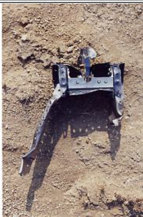
X-15 FLAP HINGE FRONT AND REAR VIEW OF A TITANIUM FLAP ATTACHMENT HINGE THAT WAS TWISTED AWAY FROM THE X-15's WING AS THE FLAP WAS TORN APART AT SPEEDS IN EXCESS OF 2,000 MPH
