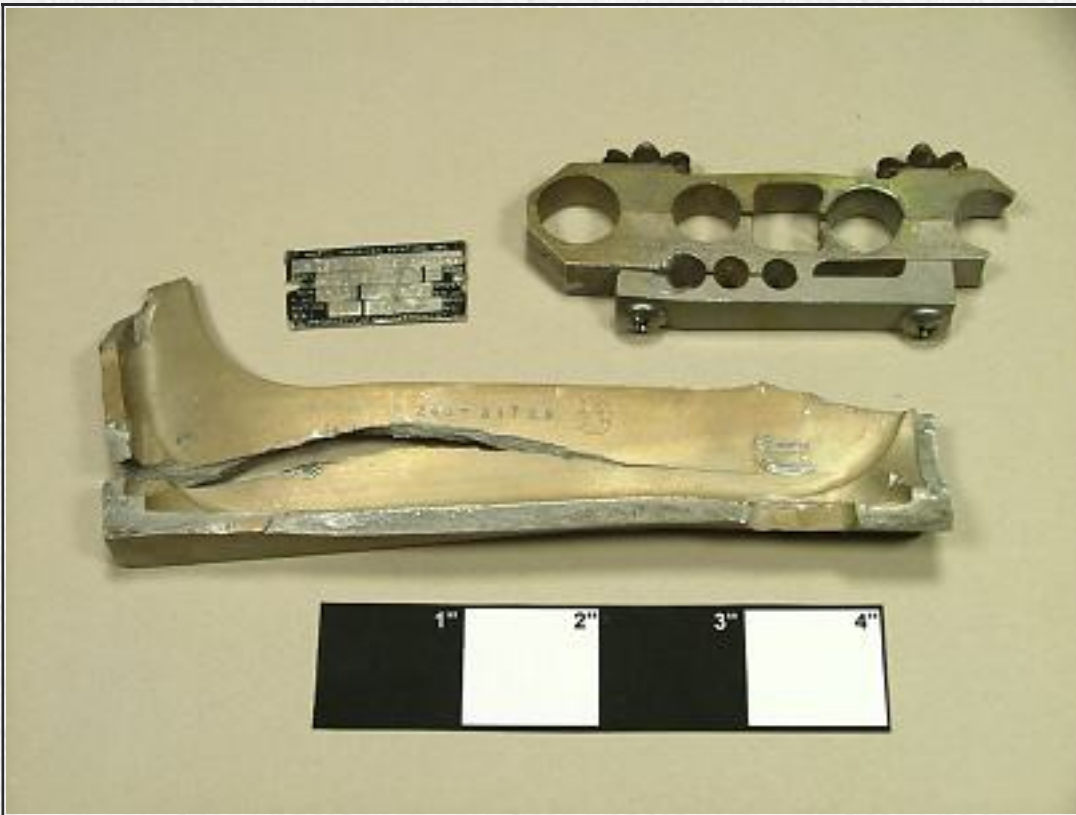
X-15 PART NUMBERS & INSPECTION STAMPS SEVERAL PARTS SHOWING NORTH AMERICAN AVIATION MANUFACTURER INSPECTION STAMPS AND PART NUMBERS. THESE ARE USED TO CONFRIM THE AIRCRAFT'S IDENTIFICATION
