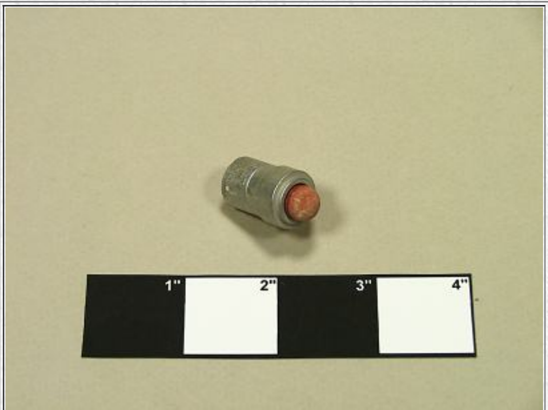
X-15 PILOTS MIC SWITCH THIS MICROPHONE SWITCH WAS LOCATED ON THE X-15's STICK GRIP. THUMB ACCUATED, IT WAS USED BY THE PILOT TO COMMUNICATE
