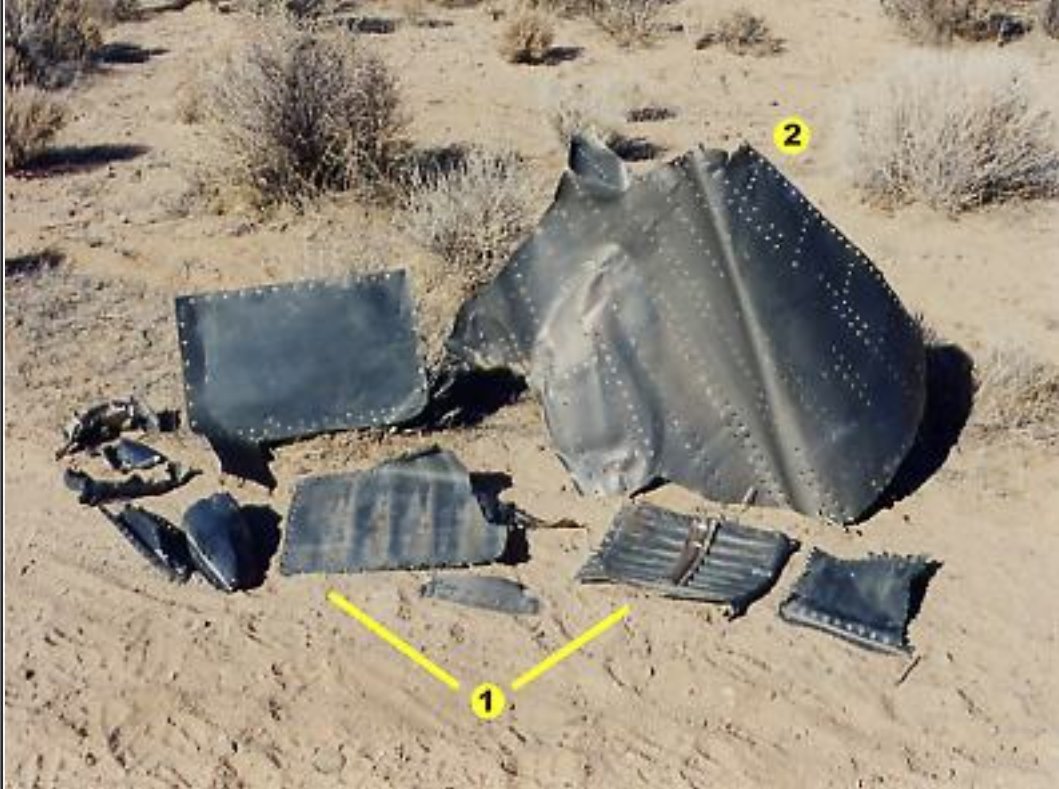
X-15 FUSELAGE PIECES 1. VARIOUS AIRCRAFT PANELS AND DEBRIS BLOWN OFF THE FUSELAGE AS IT BROKE UP 2. LARGE SECTION OF INCONEL-X WING SKIN RIDDLED WITH HOLES CREATED WHEN IT WAS TORN AWAY FROM THE RIVETS HOLDING IT TO THE WING'S STRUCTURE AT SPEEDS IN EXCESS OF 2,000 MPH
