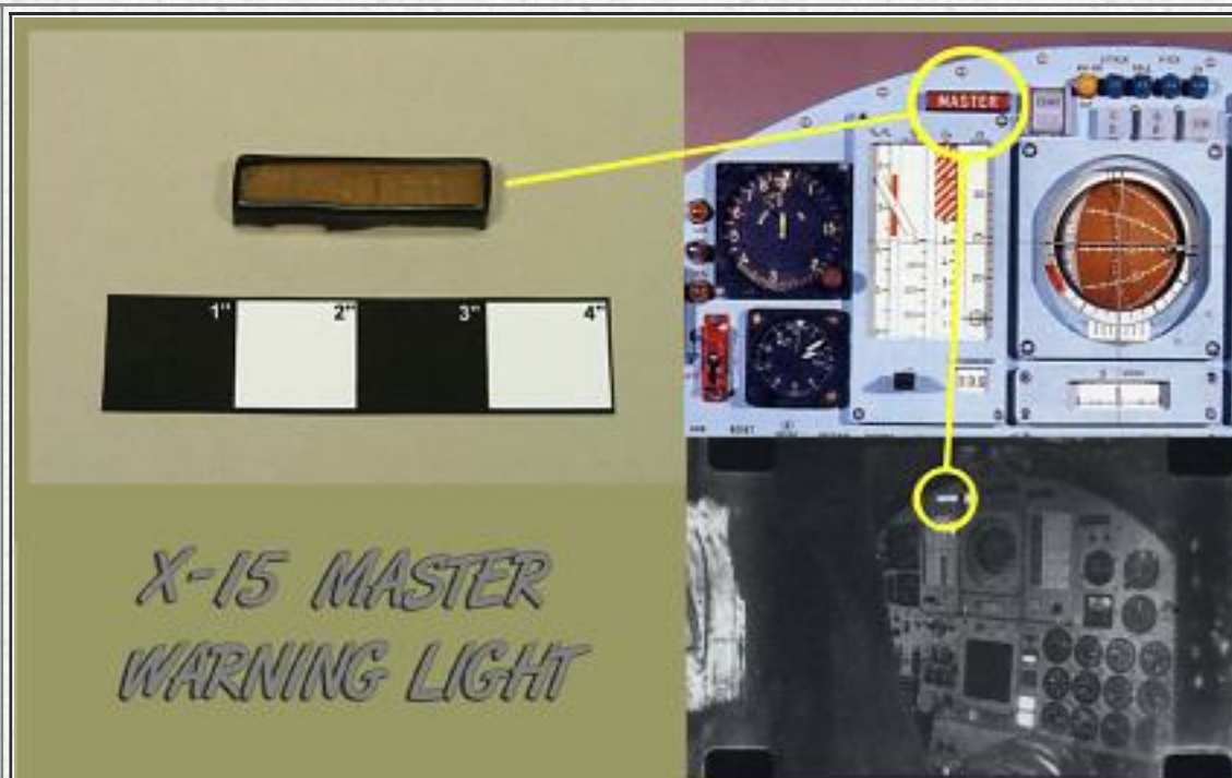
X-15 MASTER WARNING LIGHT THIS MASTER WARNING LIGHT WAS LOCATED ON THE UPPER LEFT SIDE OF THE #3 X-15's MAIN INSTRUMENT PANEL (CIRCLED IN THE UPPER RIGHT PHOTO). THE LIGHT ALERTED THE PILOT TO ANY CRITICAL FLIGHT SYSTEM PROBLEMS AND CAN BE CLEARLY SEEN ILLUMINATED IN ONE OF THE LAST FRAMES OF THE COCKPIT CAMERA'S FINAL FOOTAGE. (CIRCLED IN THE LOWER RIGHT PHOTO)
