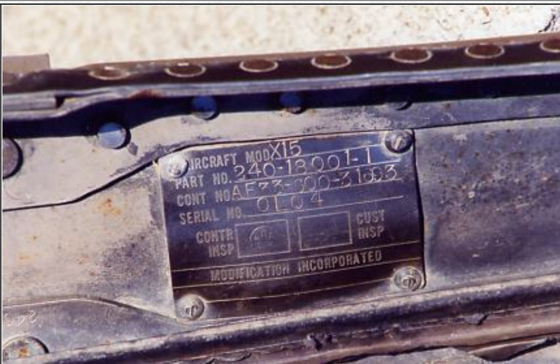
X-15 AIRCRAFT DATA PLATE CLOSE UP OF AN AIRCRAFT DATA PLATE ATTACHED TO WHAT WAS ONCE THE INNERMOST STRUCTURAL EDGE OF THE RIGHT WING FLAP. ON IT CAN BE SEEN THE DESIGNATION "X-15", THE AIRCRAFT'S PART NUMBER AND A NORTH AMERICAN AIRCRAFT INSPECTION STAMP THAT MADE THIS ARTIFACTS IDENTIFICATION RATHER EASY
