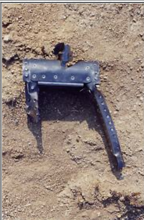
X-15 FLAP HINGE FRONT AND REAR VIEW OF A TITANIUM FLAP ATTACHMENT HINGE THAT WAS TWISTED AWAY FROM THE X-15's WING AS THE FLAP WAS TORN APART AT SPEEDS IN EXCESS OF 2,000 MPH
