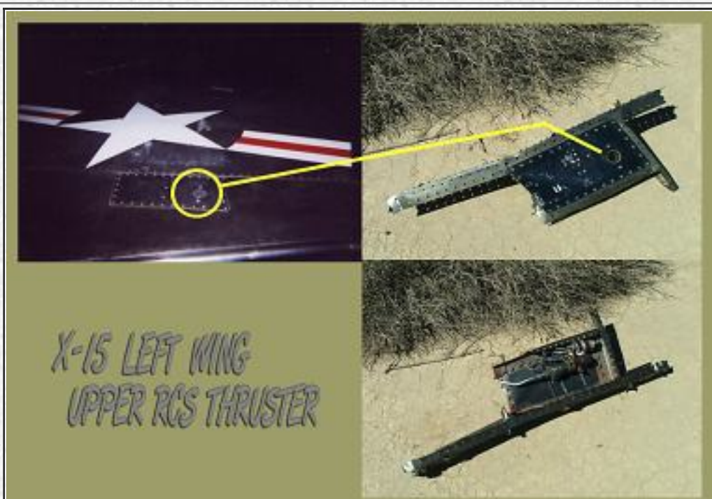
X-15 RCS THRUSTER THE PHOTOS ON THE RIGHT SHOW A TOP AND BOTTOM VIEW OF ONE OF THE X-15's REACTION CONTROL SYSTEM THRUSTERS THAT WERE USED TO CONTROL THE VEHICLE WHILE IN THE VACUUM OF SPACE. THIS ONE, ONCE MOUNTED IN THE UPPER SIDE OF THE LEFT WING IS IDENTICAL TO THE ONE IN THE PHOTO OF THE #2 X-15's WING SHOWN ABOVE. THE THRUSTER ASSEMBLY IS STILL ATTACHED TO A SECTION OF THE WING'S STRUCTURE AND, IF YOU LOOK CLOSELY, REMNANTS OF THE WHITE "BEWARE OF BLAST" WARNING PLACARD CAN BE STILL BE SEEN NEXT TO THE THRUSTER'S NOZZLE
