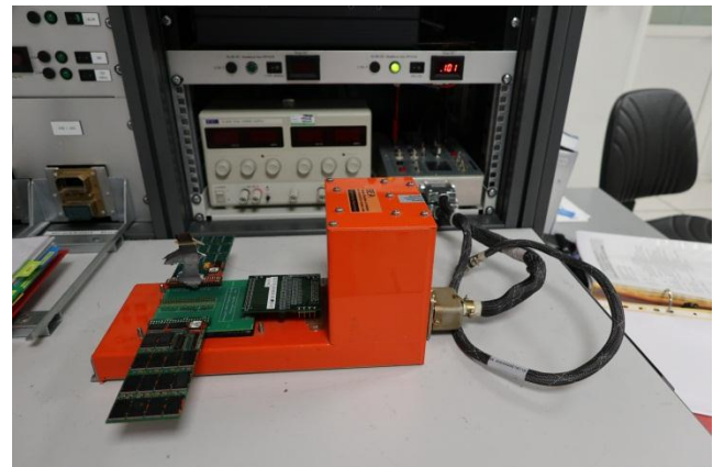
Fig 20 : CVR circuit boards on a golden chassis for readout
