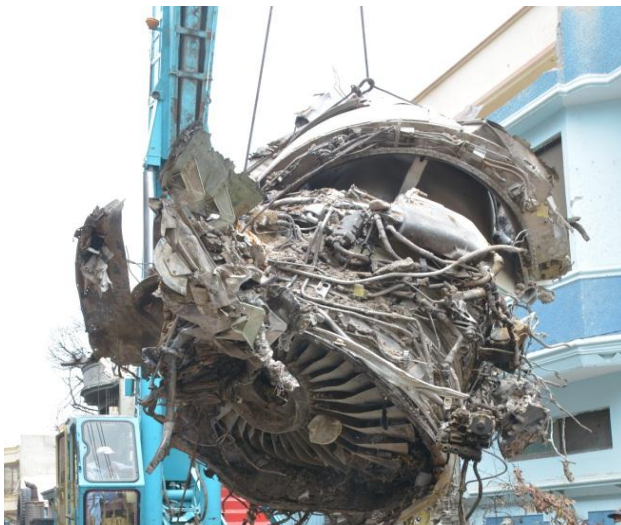
Fig 9 : Left engine being lifted from roof top
