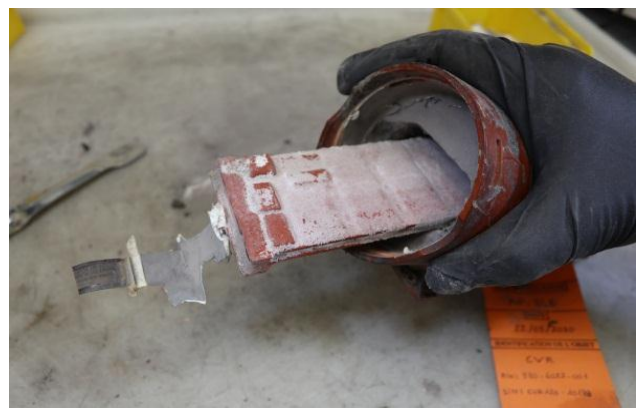
Fig 18 : CVR opening for data recovery
