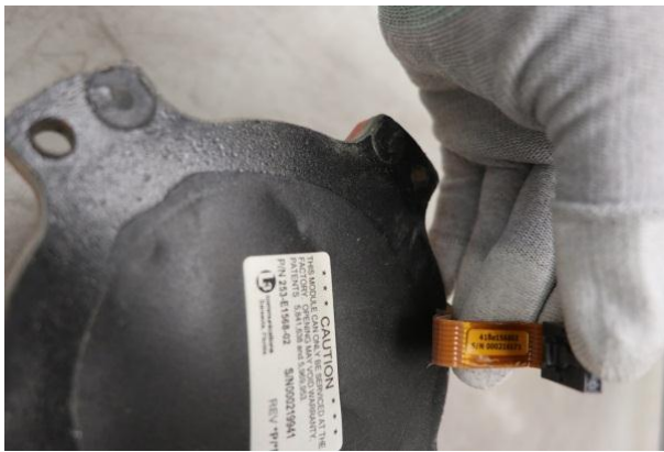
Fig 17 : FDR opening for data recovery
